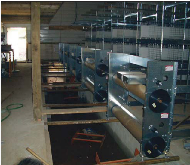
Enriched colony systems all utilize manure belts that limit the length of these systems to approximately 550 feet. Photo courtesy of North-east Agri Systems
